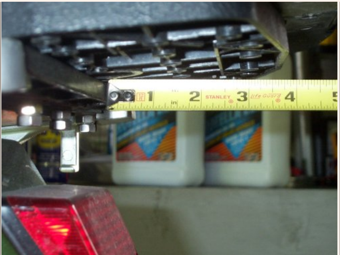
The picture above shows the back end of the stock KLR rack being measured to the middle-end of the mounting plate. This measurement is 3 3/4"
