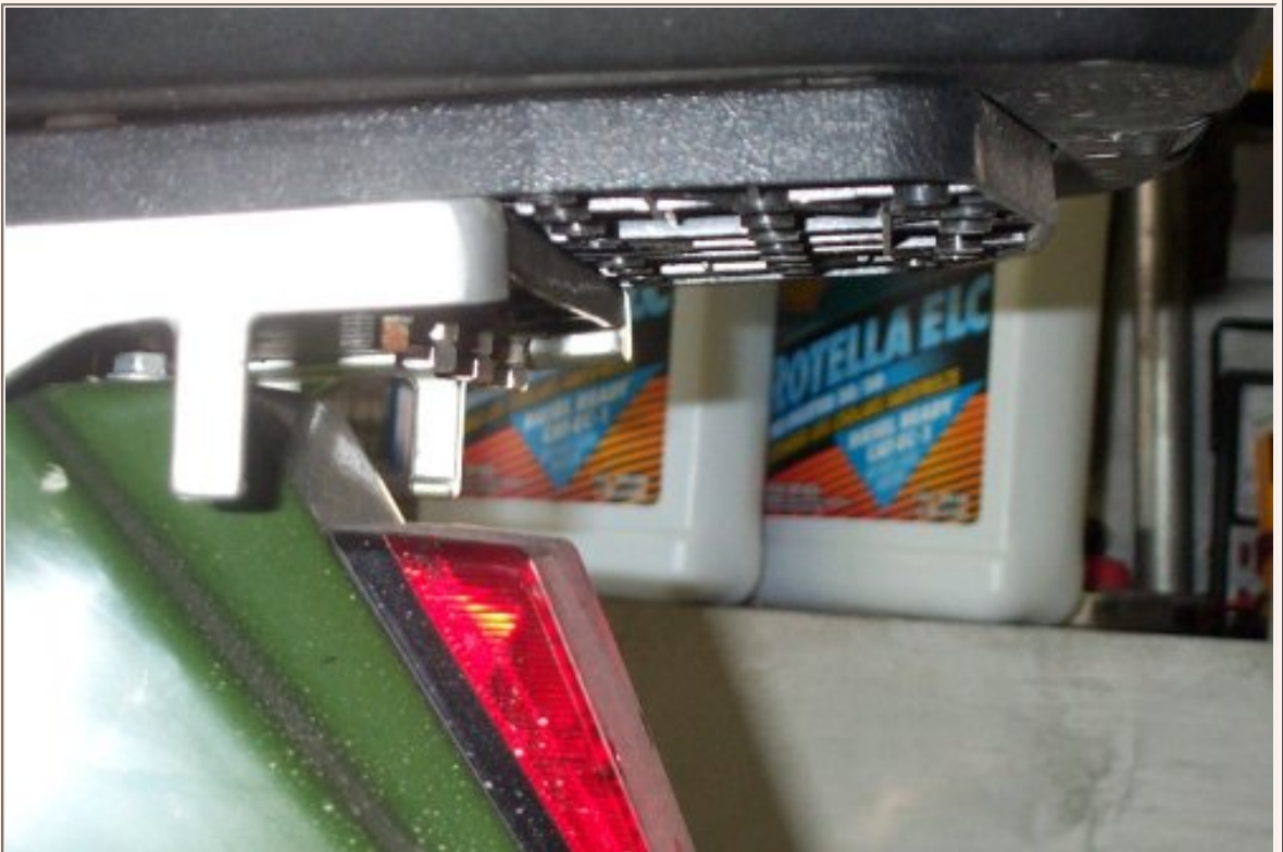
The picture above shows the back end of the stock KLR rack being measured to the middle-end of the mounting plate. This measurement is 3 3/4"
