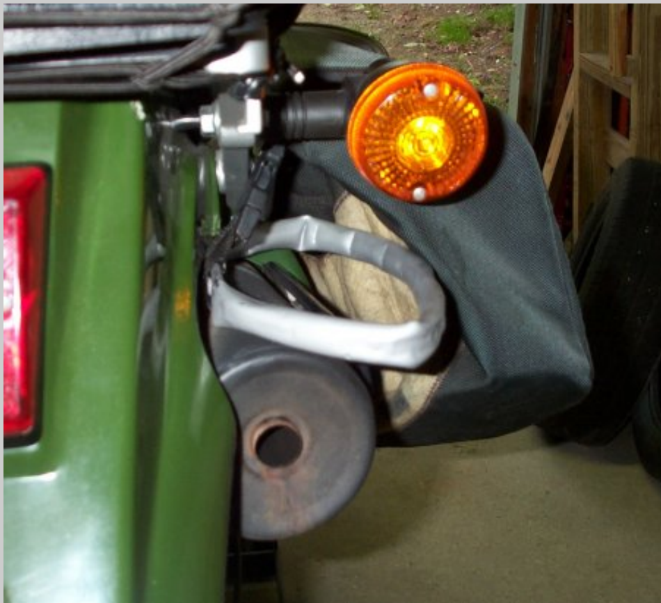
Last but not least, the picture above shows that the EMT rack is doing a good job of keeping the saddlebag away from the muffer.
