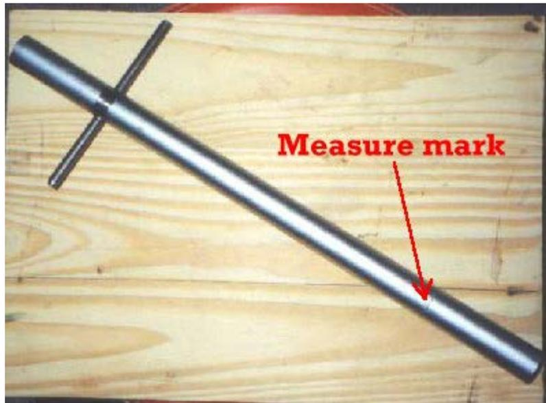
**Make sure to drill the hole through the tube perfectly level**, or the measurement will be off. The score near the bottom of the tube, which is the actual measuring mark, was made with a tubing cutter.
