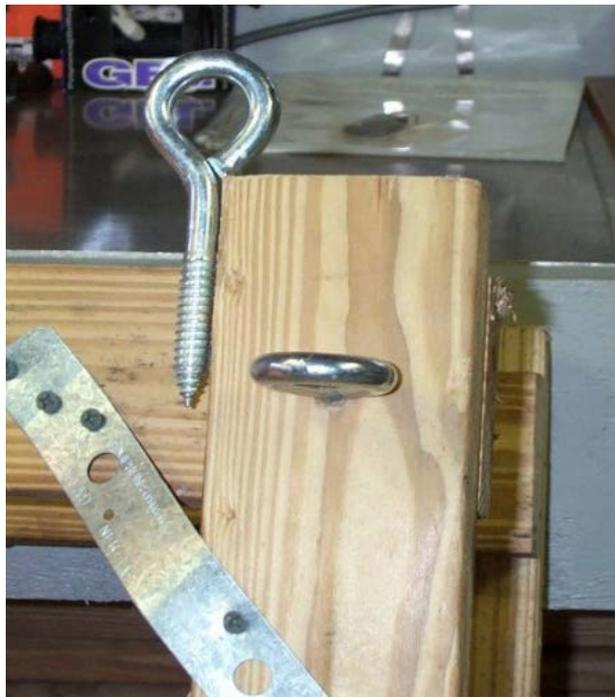
I realized that if there was vigorous work to be done on the bike while on this lift, it probably wouldn't be as stable as it should be. To improve the situation, I screwed a heavy-duty eyebolt (shown above) on both sides of the lift where the "arm" meets the upright support.
