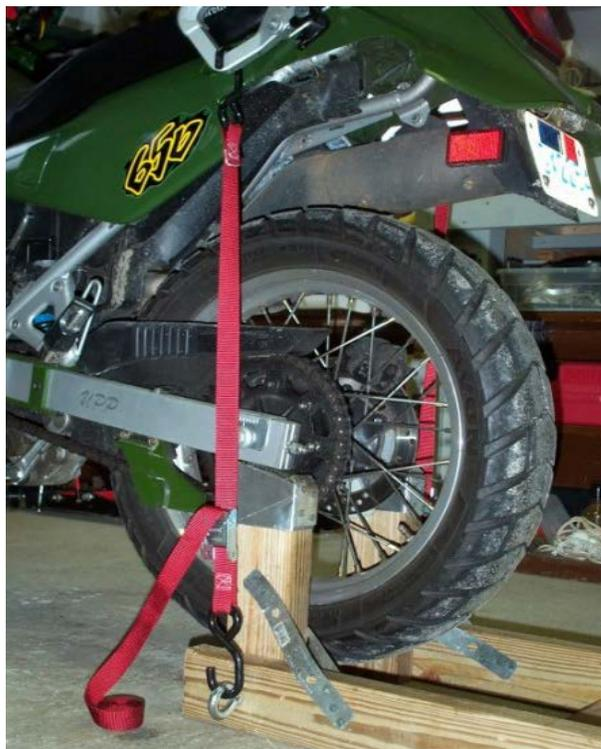
As shown above, I just run ratchet ties from the eyebolts to the bottom of the passenger grab handle. You can even put a weight on the end of the lift, if you want.
