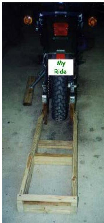
**Parts.** 3 pressure treated 2x4's, 4 strap braces (Home Depot / Simpson LSTA9), 1 45 degree brace (Home Depot / Simpson A33), galvanized course thread deck screws, and a couple strips of rubber for the tops of the uprights.
