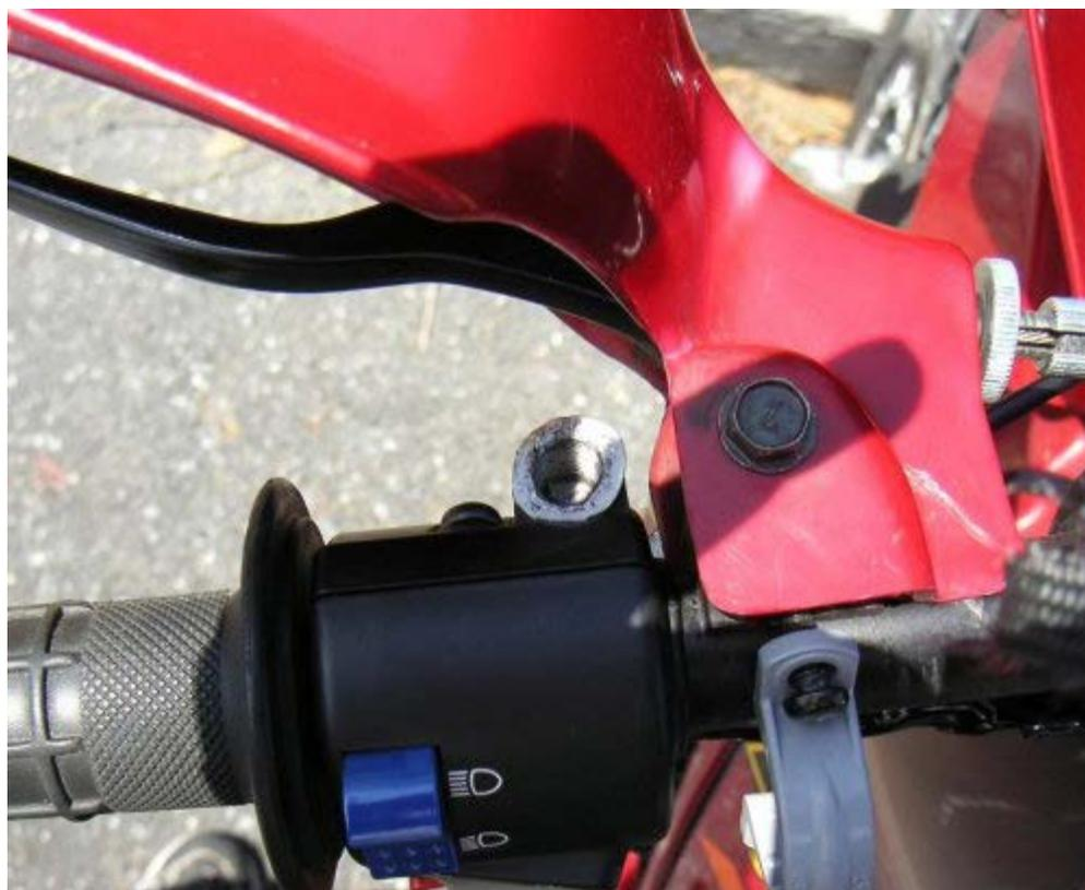
First, I had to find a bolt the same thread as the mirror, which is M10x1.25. The bolt just needs to protrude through the broken piece and
