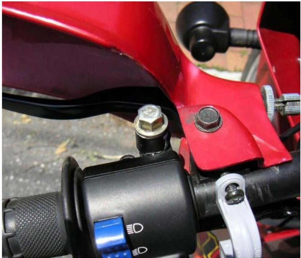
When the epoxy is dry unthread the bolt and thread the mirror in using Loctite. Presto, it's fixed! The epoxy is sandable and paintable for the meticulous types.
