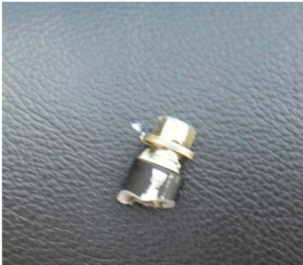
Then mix 2 part epoxy and apply sparingly to both the base and the broken off part.
