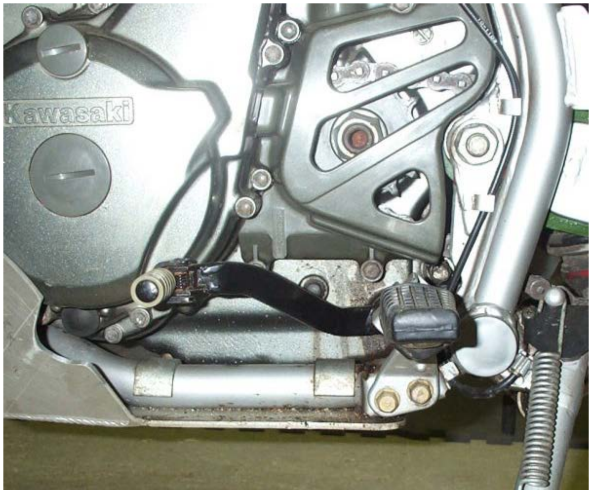
This is the IMS shifter mounted on my KLR. (That's not a countershaft seal leak, just a heavy-handed application of WD40)
