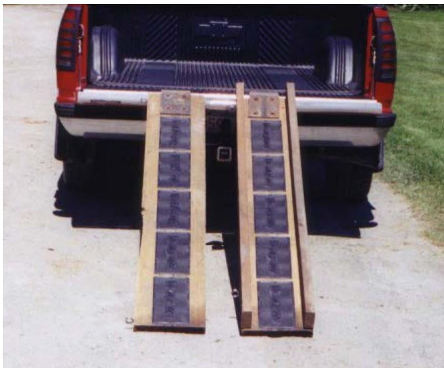
The picture above shows the ramps set up on the tailgate of my truck, and ready to go. I used two 2x12 pressure treated boards for the ramps, and to the one shown on the right, screwed two 2x4's on edge along the whole length of the ramp. This keeps the tires from wandering off the side. Each ramp is 6 feet long.
