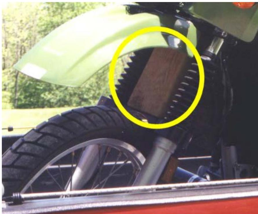
The picture above shows a 4x4 block set between the Superbrace and the top of the fender. I've read that it may be possible to strap down the front end so much that after bouncing around for a while in that position, the fork seals may blow. I don't know if this is a valid concern
