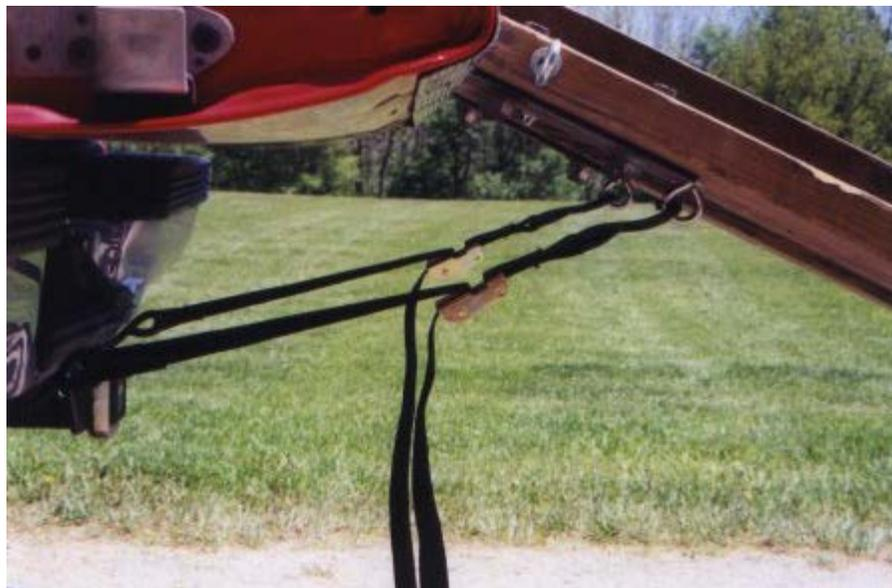
The above picture shows the use of tie-down straps to hold the ramps "into" the tailgate. \*I\* think this is a very important thing, as it prevents the ramps from kicking out or being knocked off / sideways. I just screwed a couple heavy eyebolts to the underside of the ramps, and ground off what little came through the top side.
