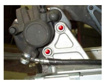
Next, remove the caliper itself by taking out the mounting bolts, shown in the picture above, marked by red dots. I suggest removing the bottom bolt first, and then holding the caliper as the top bolt is removed.
