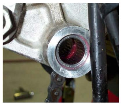
There are four areas where the bearings are to be found, as shown in the two pictures above. They are the two ends of the swingarm, and in the middle underneath where the top of the links connected. The fourth is part of the shock mount, and where the bottom of the links connected.
