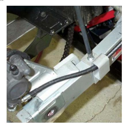
The order in which you do this, wheel or caliper doesn't really much matter, but I prefer to remove the caliper first. As shown above, remove the brake line holder.
