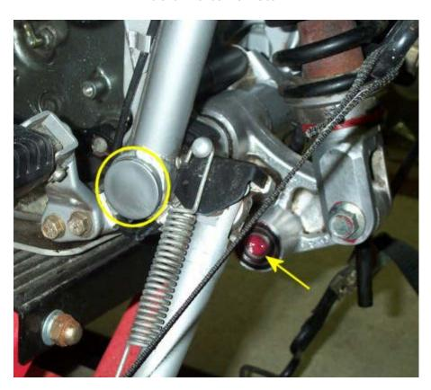
Remove the gray caps on either side of the bike, (circled), and then remove the bolt. I had to use a very long screwdriver to tap the bolt all the way through.
