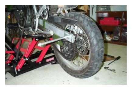
To avoid re-adjusting your chain, loosen the axle nut, and remove the axle. Slide the wheel forward until you can take the chain off the rear sprocket. Then, remove the wheel.
