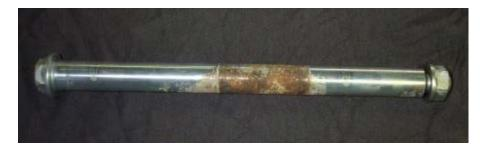
This is what I found when the bolt was removed. It came out alright now, but in another couple years I bet it would have caused some real trouble. I cleaned it up, and greased it before reinstalling.
