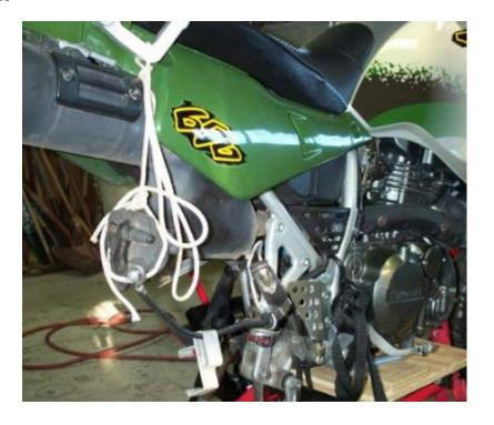
Hang the caliper out of the way, or place it on something like a 5 gallon pail - don't allow it to just hang by the brake line.
