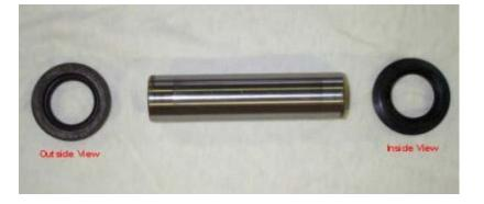
The picture above shows the shaft and seals. All bearing locations have this arrangement, but the shafts are shorter on the two swingarm ends.
