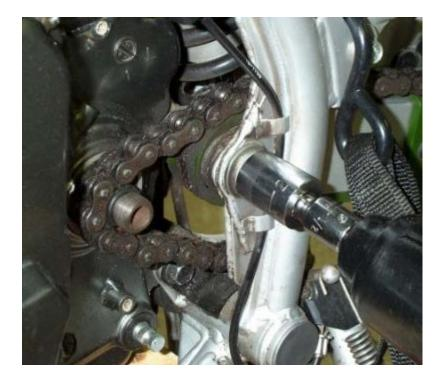
Next is to remove the main mounting bolt. This one can be troublesome if you've neglected to perform this service. There are a multitude of options; some people just whack the bolt end with a mallet, or, as I suggest trying, with the nut removed, put an impact socket on the bolt head and let it hammer away until the bolt breaks free of the corrosion.
