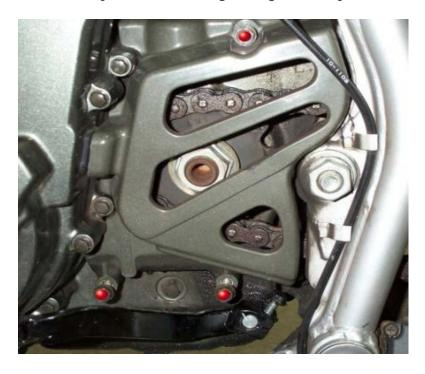
Next, remove the engine sprocket cover. The position of the three bolts to be removed are marked by the red dots.
