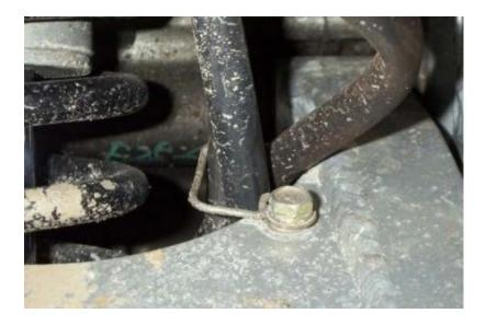
Shown in the picture above is a hose holder fastened to the upper right corner of the swingarm. You can just loosen this and take the hoses out, slip the hoses out without loosening at all, or remove the bolt and holder all together. It's easiest to just take the hoses out.
