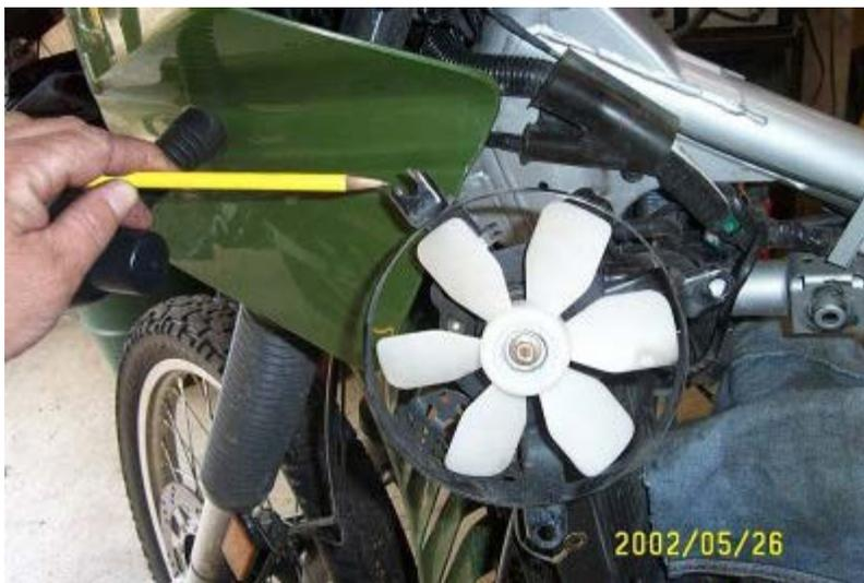
***Thanks to Dan for the picture above.*** Here's what he had to say: *The cooling fan has one bolt that is a PITA to install. By notching the hole, I leave the bolt in and just slide it into place.*
