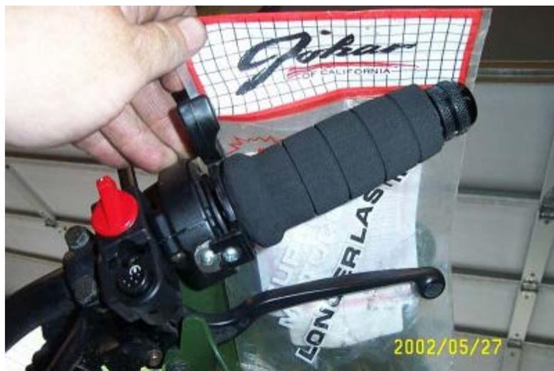
**Thanks to Dan for the above photos.** Here's what he had to say: *I didn't think the lever stuck over far enough over the throttle housing. I used a small scrap of heavy gage stainless sheet metal. Drilled one hole so a 6-32 screw would fit loose then tapped a 6-32 hole into the throttle*
