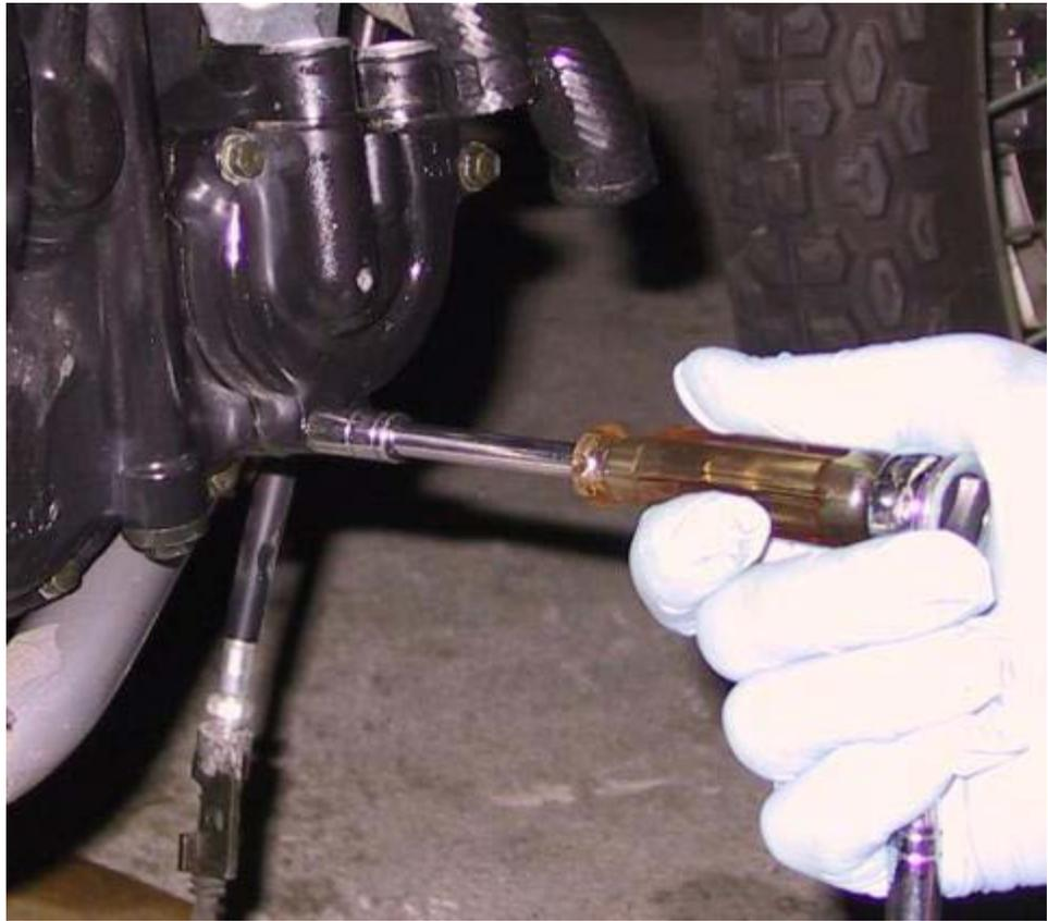
4. Remove the impeller - but **BE GENTLE!** The waterpump shaft is easy to break and expensive to fix. The impeller is held on the shaft by a small nut (10mm head) and washer. After removing the nut and washer, remove the impeller by rotating it slowly counterclockwise while pulling it off.
