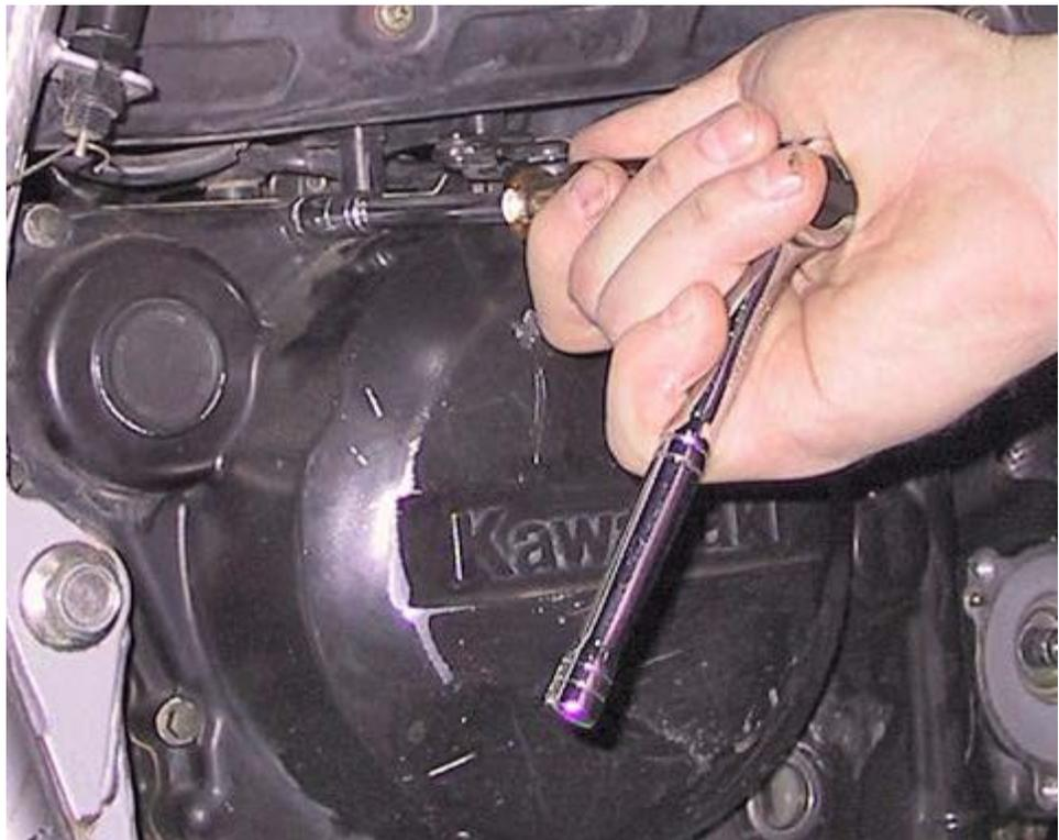
**6. Seal removal:** I made my own seal puller using a threaded bolt (3.5 in by 5/16 in), a few washers, and a couple of sockets (if you have or can borrow a seal puller, so much the better). First, put a small flat washer on the bolt, and then insert it from the inside of the case through the oil seal and mechanical seal.
