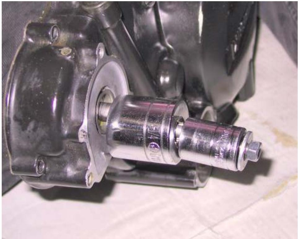
**NOTE: Be careful here, if the inside washer hangs up on the case, you can damage the engine cover \$\$\$.** Make sure the washer you're using fits up
