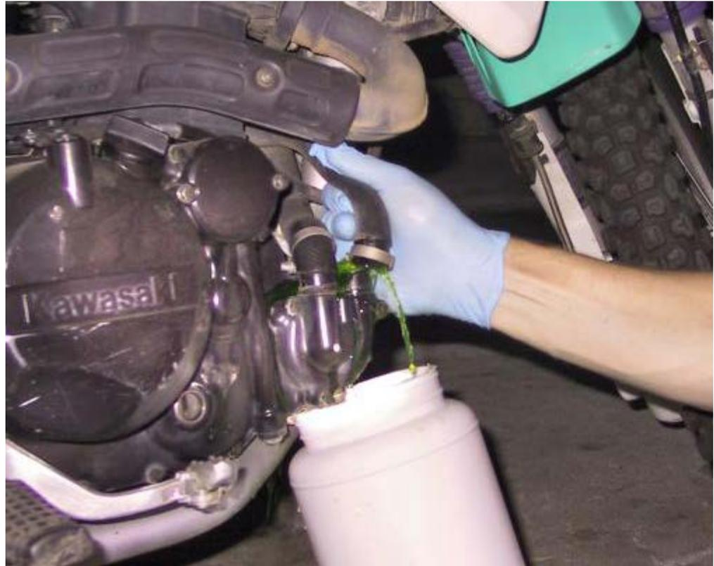
**3.** Next, remove the water pump cover (3 screws, (2) 6mm x 30mm, and (1) 6mm x 35mm, all with 8mm heads). Take a moment here to inspect the hoses for wear or cracking and replace as needed. The stock hose set will cost about \$60 from the dealer, but a Goodyear #63936 heater hose can be cut to fit all three pieces and costs about \$25. Replacement hose clamps are also available from your local auto parts store.
