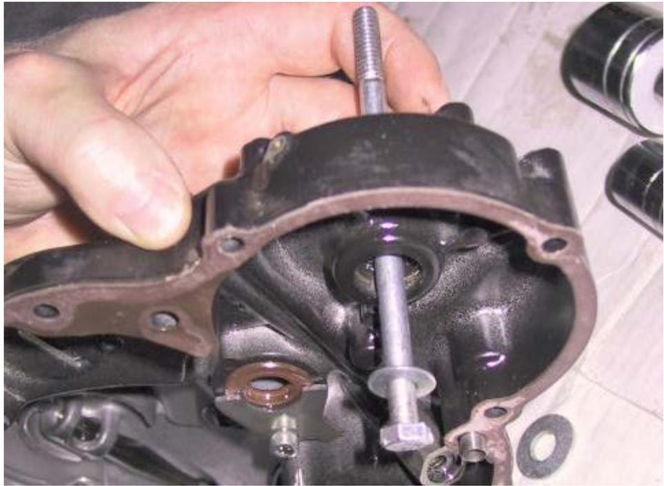
...then put a large socket (24mm or a 1 & 1/4 inch, 1/2inch drive socket) and a couple of washers on the outside of the bolt where it sticks through the case (these are just spacers). You need to use a socket large enough for the mechanical seal to easily slide into. Put the nut on the end of the bolt and tighten it up.
