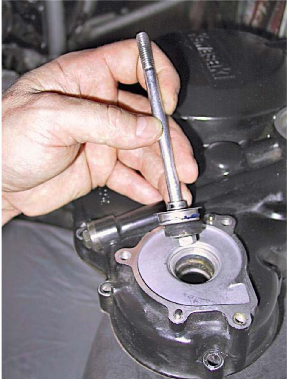
**7.** The other half of the mechanical seal is in the back of the impeller. It can be gently pried out with a small screwdriver (jewelers). Take care not to mar or scratch the impeller.
