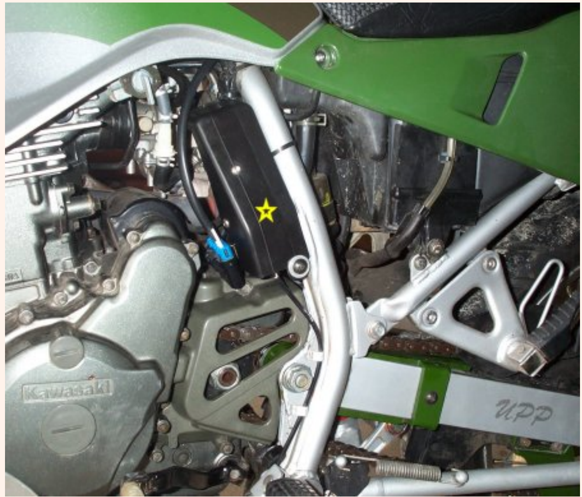
The two fuse blocks included in this kit will be placed inside the sidestand switch cover, indicated in the picture above by the yellow star.
